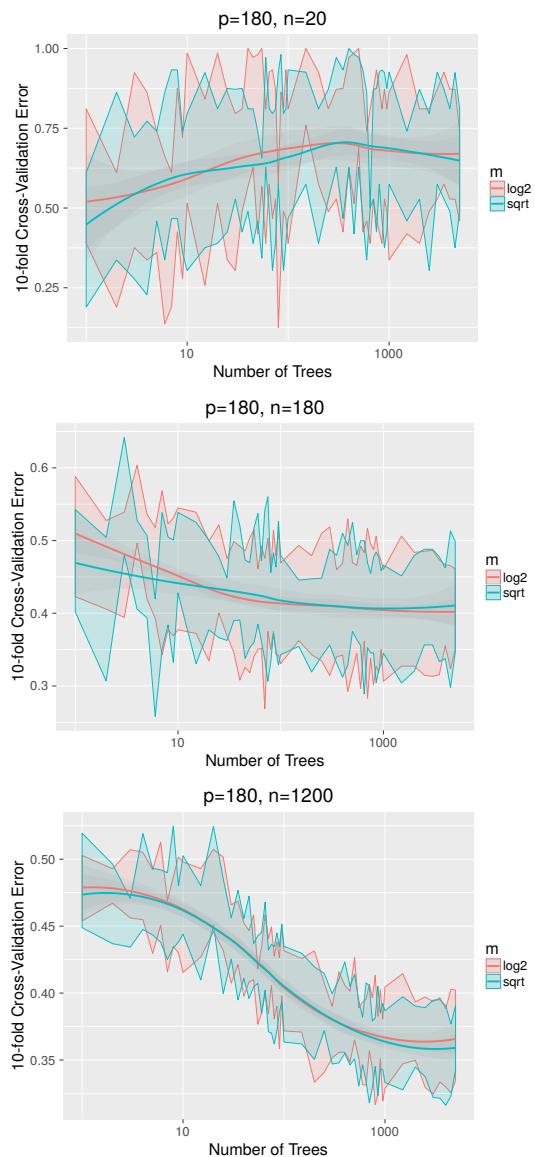
Figure 2. 10-fold cross validation error for three cases of n , the number of trees, and p , the number of predictors. The shaded regions represents the 95% ( 2\hat{\sigma} ) confidence interval on the mean.
